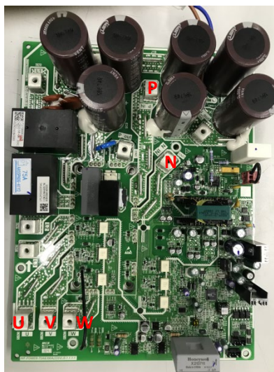
Figure 6-2.1: Inverter module terminals
