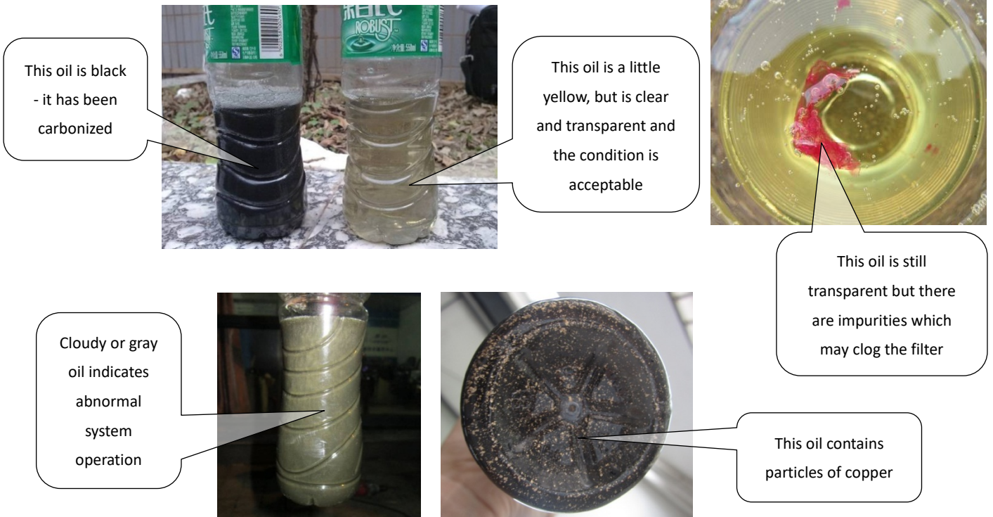
Figure 6-2.10: Inspecting compressor oil
