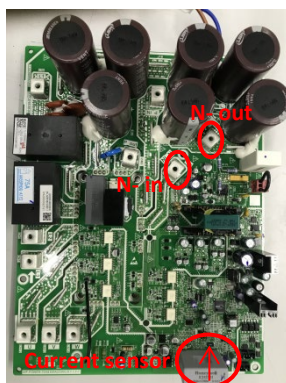
Figure 6-2.5: DC detection wire connection method
