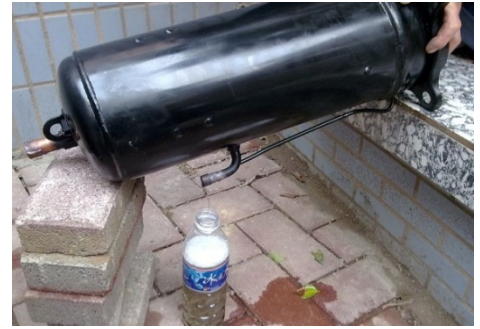
Figure 6-2.8: Draining oil from a compressor
