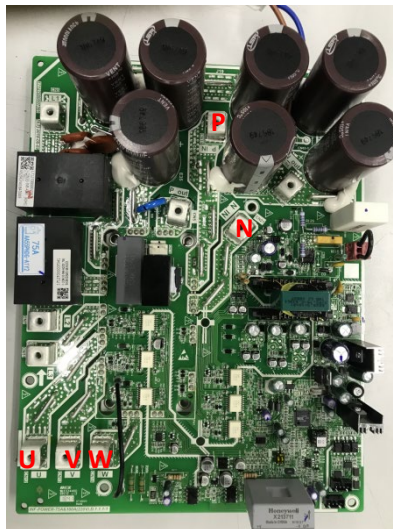
Figure 6-2.6: Inverter module terminals
