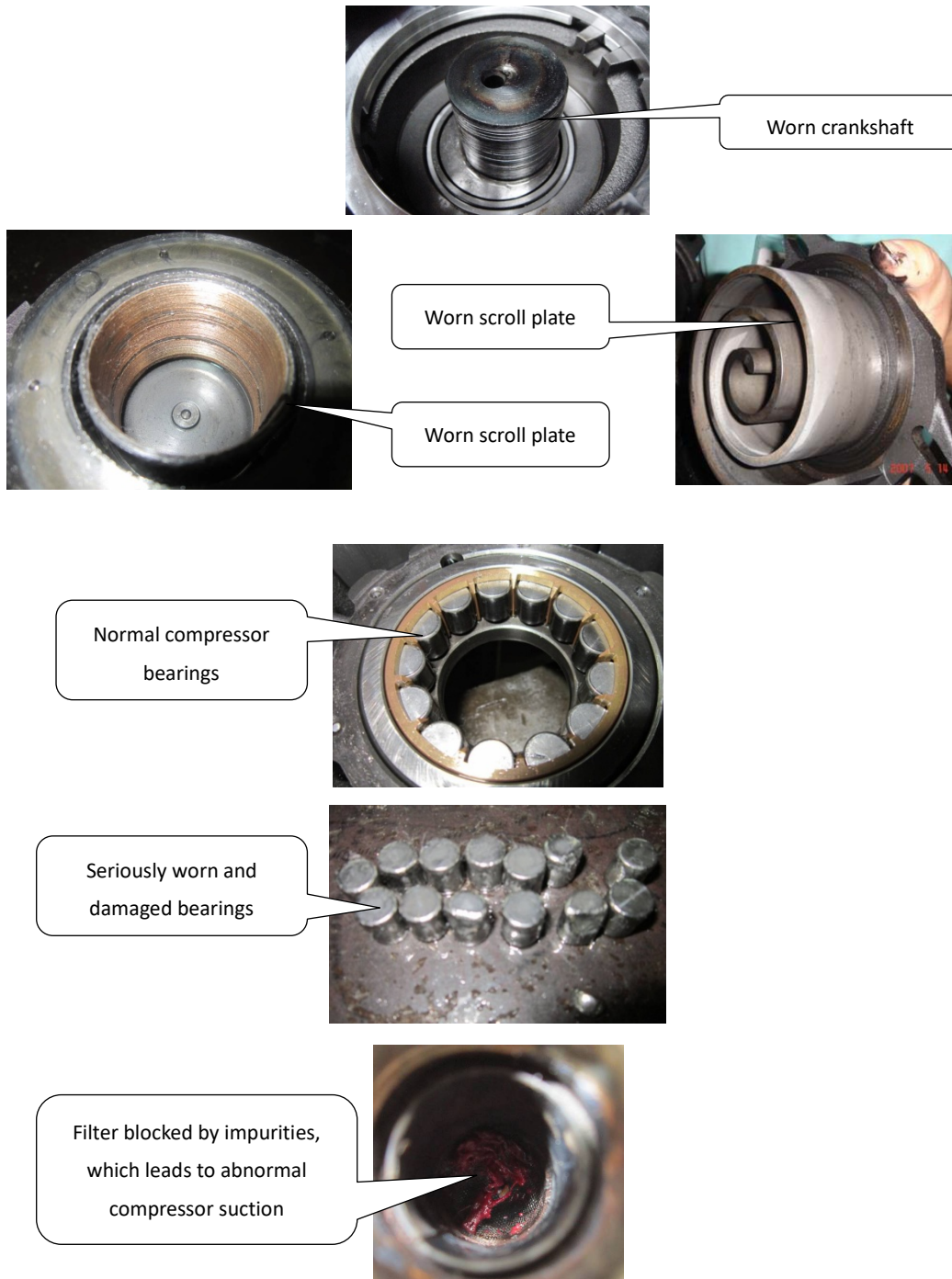
Figure 6-2.11: Effects of spoiled compressor oil
