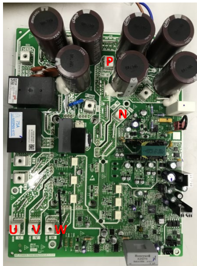
Figure 6-2.7: Inverter module terminals
