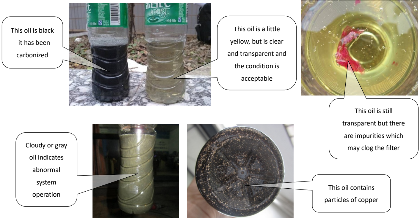
Figure 6-2.10: Inspecting compressor oil
