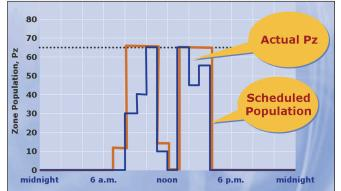
Figure 5 (left): Sensed presence profile. Figure 6 (right): Scheduled occupancy profile.
