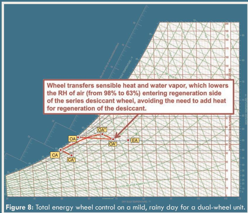
Figure 8: Total energy wheel control on a mild, rainy day for a dual-wheel unit.
