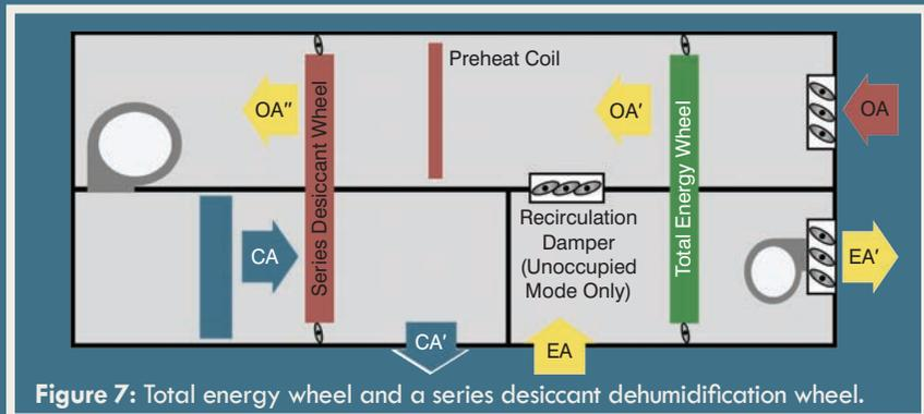
Figure 7: Total energy wheel and a series desiccant dehumidification wheel.
