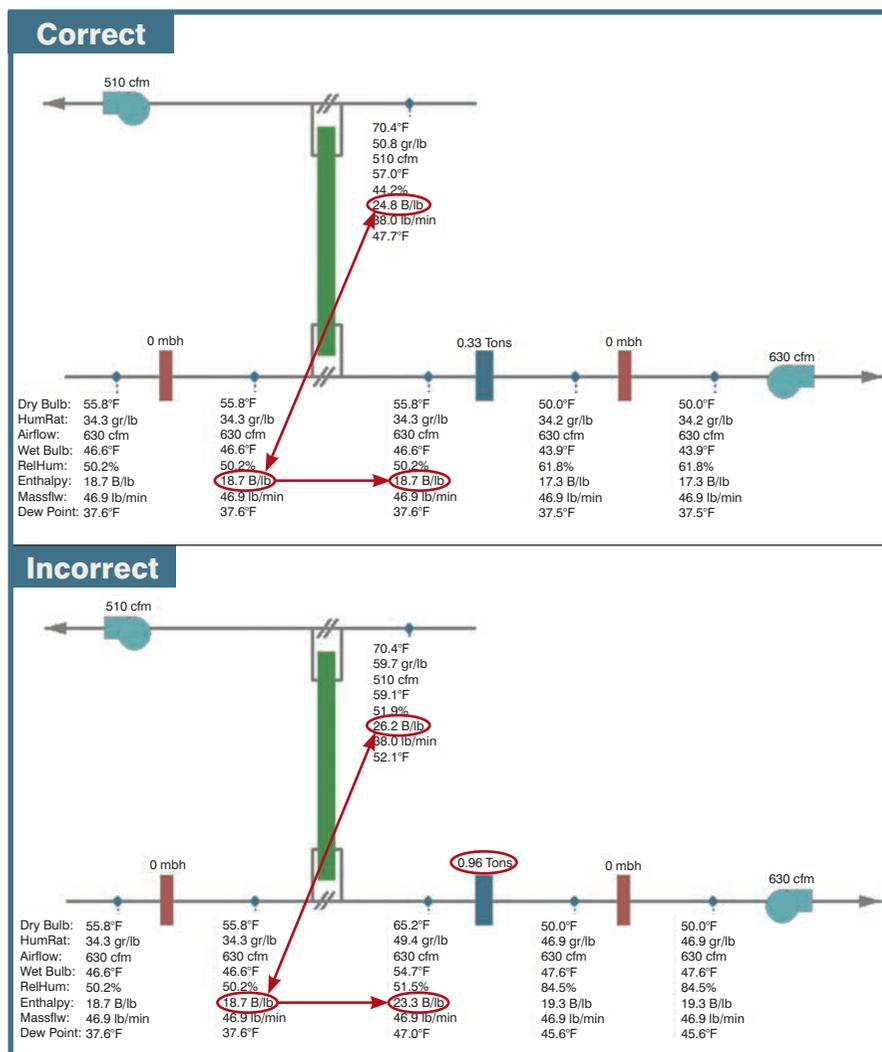
**Figure 9: Modeling on/off total energy wheel control on a mild day. Correct (top):** When  $h_{OA} < h_{EA}$  the wheel should be off, and it is off. **Incorrect (bottom):** When  $h_{OA} < h_{EA}$  the wheel should be off, but it is on. This increases enthalpy of the air entering the cooling coil, which increases the coil load.
