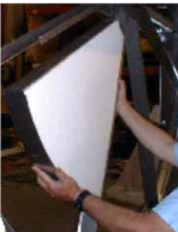
Figure 200. Slide segment on spoke until contacts stop in hub plate.
