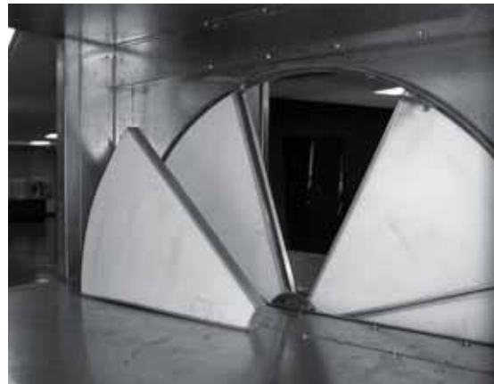
Figure 197. Insert nose of segment between hub plates to install
