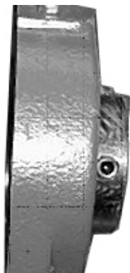
Figure 185. Loosen set screws
