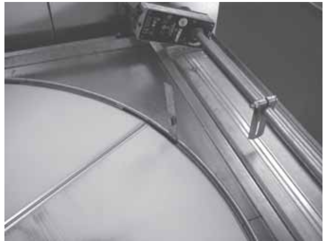
Figure 170. Completely fasten segment retainers
