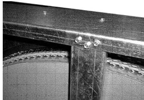
Figure 175. Remove post mounting screws
