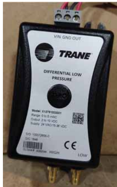
Figure 168. Fan inlet airflow measuring system
