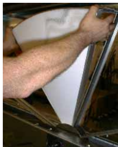
Figure 197. Insert nose of segment between hub plates to install
