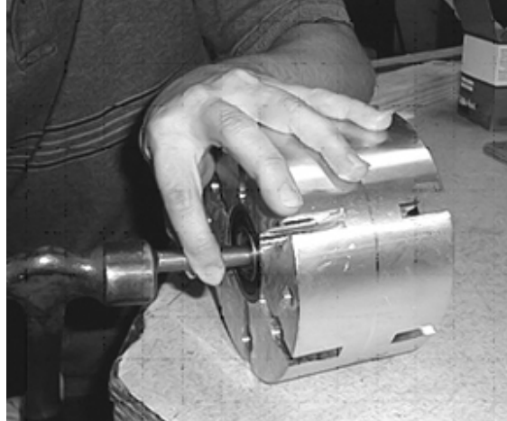
Figure 179. Remove old bearing by tapping from the back. Gently tap around the race. Repeat on opposite side.
