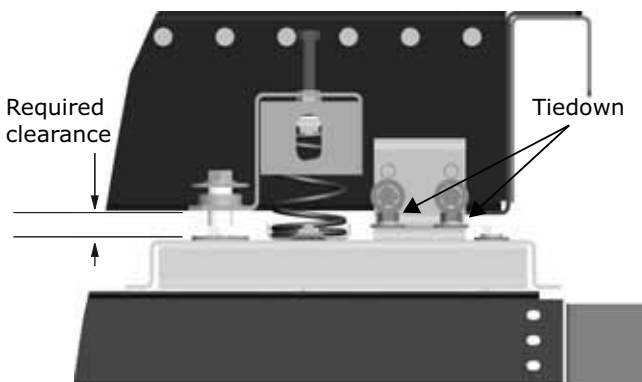
Figure 11. Isolator tie-down removal for unit sizes 35 - 120
