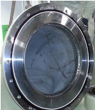
Figure 19. Installation of 1/8-in. GORE-TEX tape
