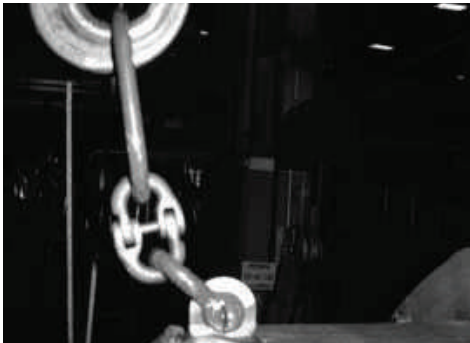
Figure 11. Lifting clevis on the suction elbow lifting tab
