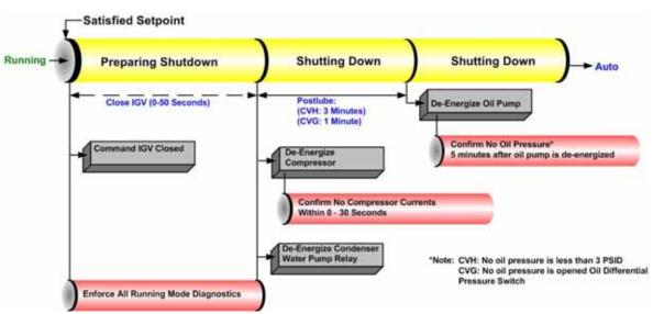
If the STOP key is pressed on the operator interface, the chiller will follow the same stop sequence as above except the chilled water pump relay will also open and stop the chilled water pump after the chilled water pump delay timer has timed out after compressor shut down (see Figure 47).
