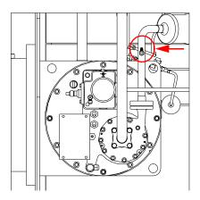
Note: The holding charge should register approximately 5 psig (34.5 kPaG) at 72°F (22.2°C). Place a gauge on the access valve provided (indicated by arrow and circle in the preceding figure) on the refrigerant pump discharge line to verify the holding charge. If the charge has escaped, contact your local Trane sales office for instructions. For Duplex™, verify charge on both units.
