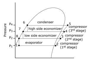
Figure 35. Refrigerant flow, 3-stage
