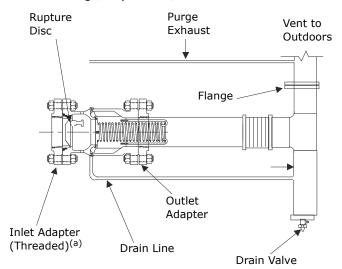
(a) The pipe-thread joint at the Inlet Adapter (Threaded) connects to the chiller and must be leak-free. For more information, refer to Installation, Operation, and Maintenance: RuptureGuard Pressure Relief System Option (CTV-SVX06\*-EN, or the most recent version).
