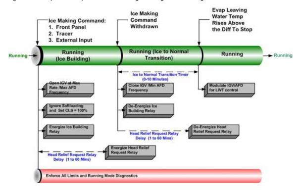
Figure 49. Sequence of operation: ice making: stopped to ice to ice building complete
