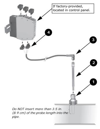
Mount the 1/2-in. NPT adapter in a horizontal or vertical section of pipe. The maximum distance from the control panel must not exceed 29.5 ft (8.99 meters) (see item labeled "1" in Figure 10, p. 20). Allow at least five pipe diameters straight run of pipe upstream of the sensor location, and three pipe diameters straight run of pipe downstream of the sensor location.
