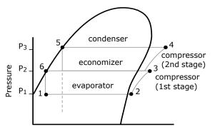
Figure 37. Refrigerant flow, 2-stage
