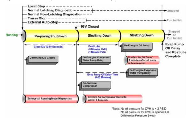
Figure 47. Sequence of operation: normal shut-down to stopped and run inhibit
