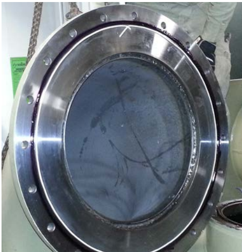
Figure 21. Installation of 1/8-in. GORE-TEX tape
