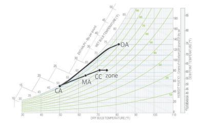
At the 45°F supply-air condition, the DOAS provides the majority of space sensible cooling and dehumidification.
