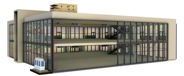
In a typical VRF system, each zone has one or more indoor units, which provide cooling and heating to maintain the desired zone temperature. As a result, a VRF system is considered a distributed HVAC system with cooling and heating equipment dispersed throughout the building.
