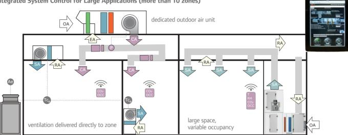
A large application may have a variety of different system types. For example, a building might utilize separate terminal and ventilation system for most zones while using a single-zone VAV (SZVAV) air handler to maintain a large space with variable occupancy, such as a cafeteria or lecture hall. The AHU is paired with a VRF heat pump condensing unit and LEV kit. A BAS can be used to coordinate all systems in the building.
