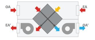
This allows the ERV to partially cool in the summer and partially heat the outdoor air in the winter. For mild weather operation, ERVs will often include an air bypass when energy recovery is not needed.
