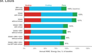
The DOAS + ERV without reheat (option 5) eliminates hot gas reheat compared to the DOAS + ERV with reheat (option 4) alternative. This comparison reveals the same recooling penalty observed when option 3 and option 2 are compared.
