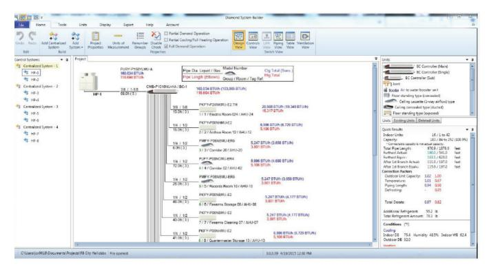
Diamond System Builder<sup>®</sup> (DSB) is the primary system design and layout tool for a VRF terminal system. The software is also used to select many of the components that make up a terminal system, or are used in conjunction with a ventilation system.
