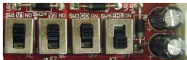
Figure 60. CSTI board-mounted switches
