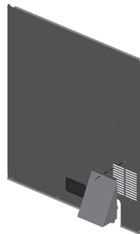
Figure 14. Vent hood installation
