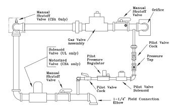
Figure 19. 235 and 350 MBH - unit gas trains (natural gas)
