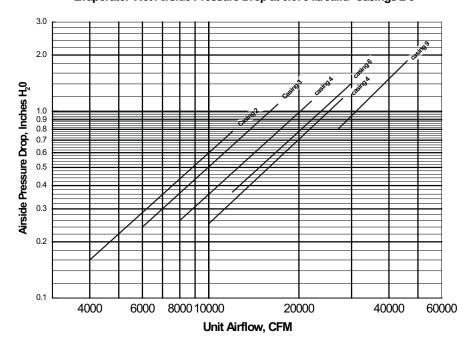
Evaporator Wet Airside Pressure Drop at 0.075 lb/cu.ft. Casings 2-9
