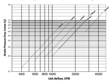
Evaporator Dry Airside Pressure Drop at 0.075 lb/cu.ft. Casings 2-9
