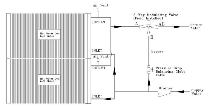
Figure 23. Hot water piping configuration for W\_HE casing 9
