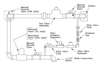
Figure 18. 500 and 850 MBH - unit gas trains (natural gas)
