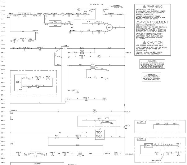
Figure 39. Typical Fenwall ignition control system
