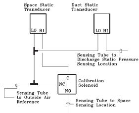
DUCT & SPACE STATIC PRESSURE CONTROL COMPONENT LAYOUT
