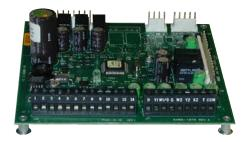
ReliaTel™ microprocessor controls are available on 3- to 25-ton units.
