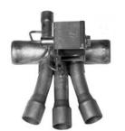
A system reversing valve (4-way valve) is included with all heating/ cooling units. This valve is piped to be energized in the cooling mode to allow the system to provide heat if valve failure were to occur. Once the valve is energized for cooling, it will remain energized until the control system is turned to the OFF position, or a heating cycle is initiated.
