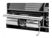
The blower housing is constructed of non-corrosive galvanized steel. Serviceability to the housing is made through the chassis air-side front panel. The fan housing is mounted onto a fan board assembly which also includes the fan wheel, and fan motor. This fan board assembly may be easily removed from the chassis by sliding the fan board frontward in maintenance or service situations.
