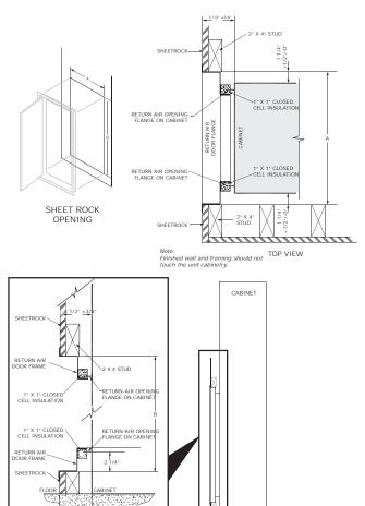
Locate dimensions A and B for sheet rock opening size. The position of the sheet rock opening must be centered side-to-side with the return-air opening in the cabinet. Ensure the bottom of the sheet rock opening is 2¼ inches below the return-air opening in the cabinet. This allows the door recess to rest on the bottom of the sheet rock opening for proper vertical placement of the door.
