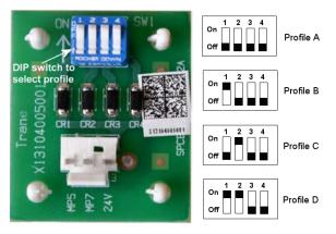
Installations at altitudes above 2000 feet may require an adjustment to the fan speed setting to achieve the proper airflow. To adjust the airflow to get the desired CFM, set the DIP switches located in the control box to the proper profile setting. Tracer<sup>®</sup> TU can be used to make further adjustments to the fan speed.
