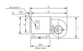
Figure 6 : HCCA Unit with Rear Return Plenum
