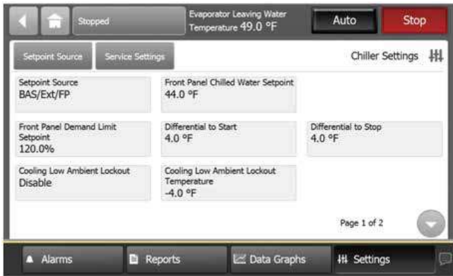
Figure 34. Equipment setting screen (Chiller setting shown)
