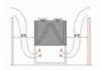
The RTAC has the smallest recommended side clearance on the market: 1.13 meters (4 feet) to maintain maximum performance. In locations where space is further limited and airflow is restricted, the RTAC will remain operational.
